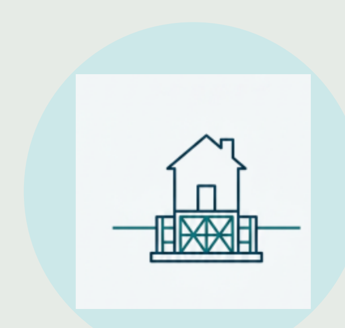
Raised, armoured foundations to protect from debris flows
