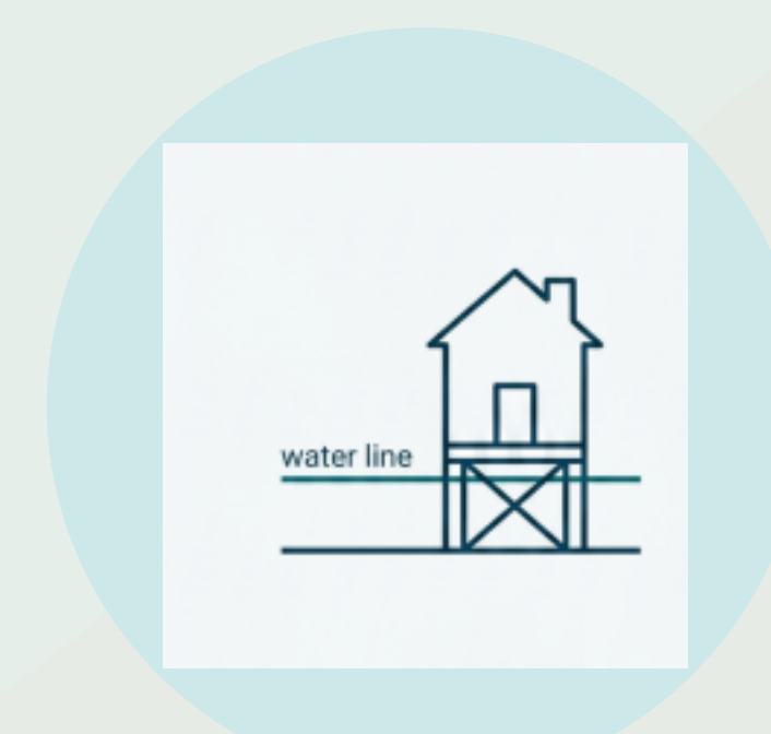
Elevating construction above flood level
