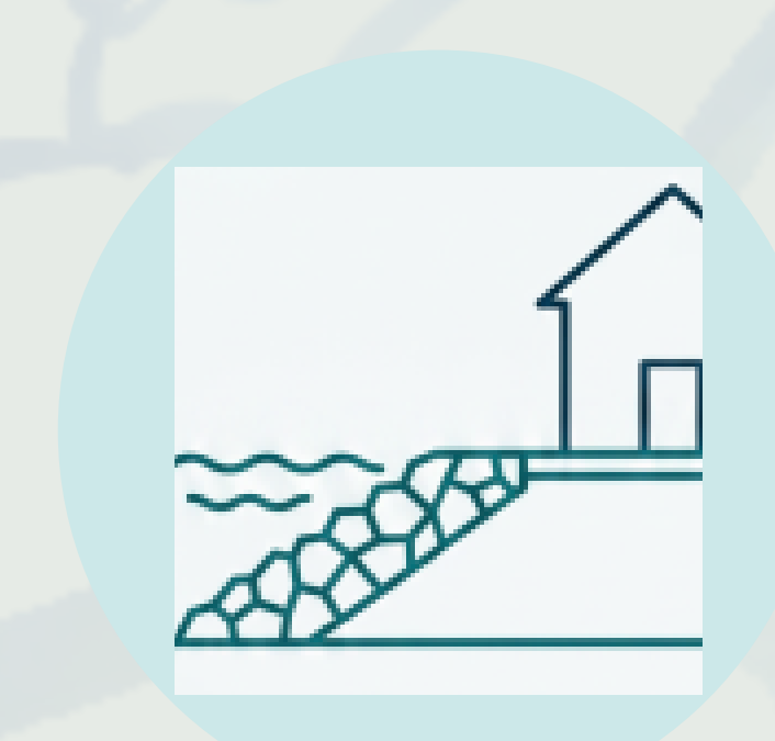
Rip-rap protection of river banks to prevent erosion
