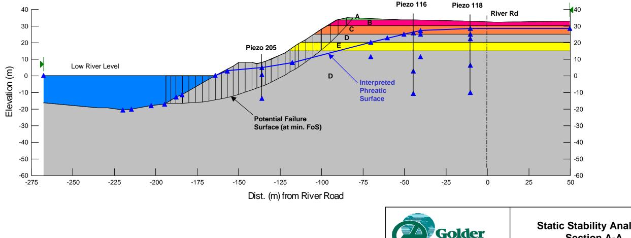
Note: Piezometer numbers referenced to Golder numbering system (for locations see Figures 1 & 2)
