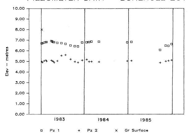
PIEZOMETER DATA - BOREHOLE 202
