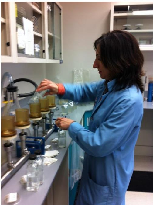
Figure 4: Metro Vancouver Laboratory technician processing water sample in preparation for coliform bacteria check
