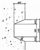
5 TYP. REVEAL DETAIL A-2 FULL SCALE
