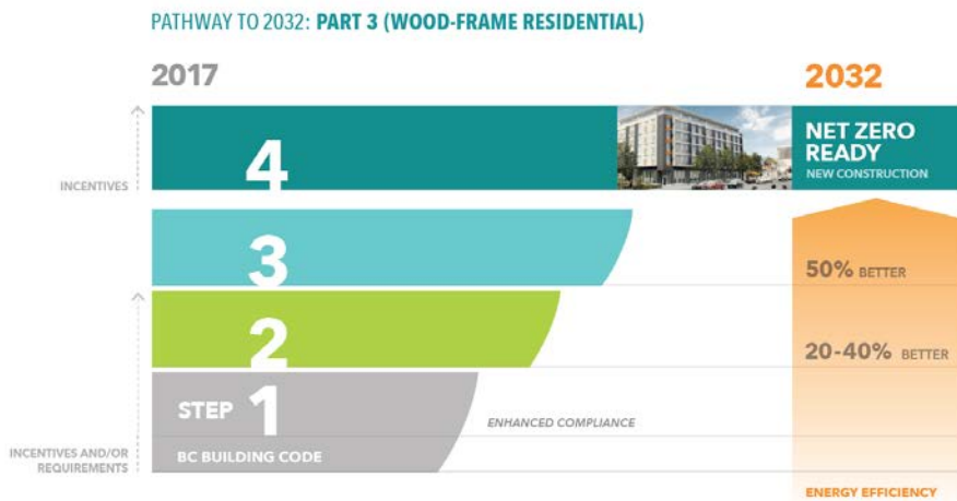
Figure 8 BC Energy Step Code "steps" for Part 3 Wood-frame Residential, as opposed to Residential Concrete or Commercial
