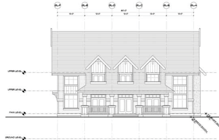
4 FRONT ELEVATION (WEST) SCALE: 1/100
